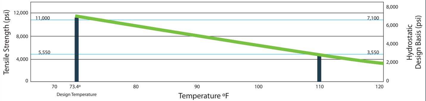
**Ductile Iron Pipe Resists Up To 5.6 Times The Hydrostatic Burst Pressure Of PVC0 Pipe**
