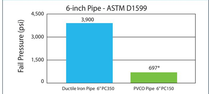
\*Burst pressure at which PVC0 pipe failed by ballooning or fracturing.
