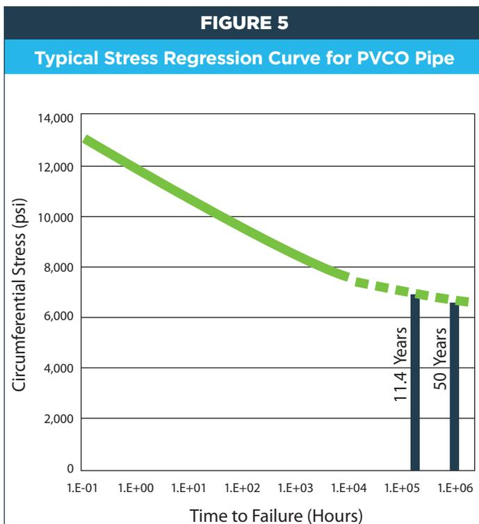
Figure 5 shows a typical stress regression curve for PVCO pressure pipe depicting the relationship between applied stress and time to failure. Note that after 11.4 years, PVCO fails under almost one-half the stress that will cause failure initially.
